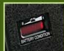
Battery Capacity Meter
